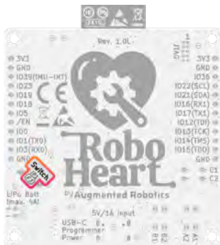
Figure 7: RoboHeart position of the SWITCH solder bridge
